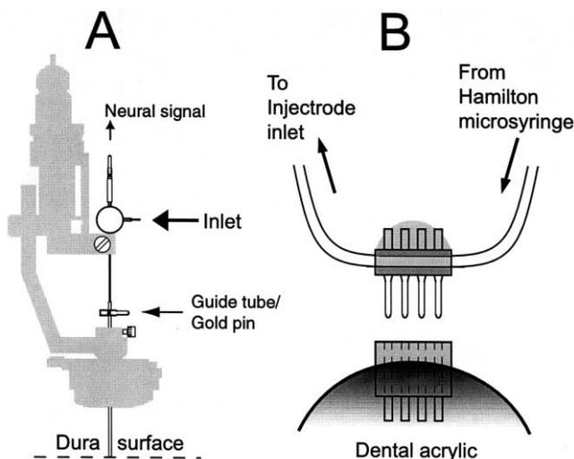
Fig. 3. Injectrode (in outlined contours) inserted through the guide tube (in outlined contours) using a micromanipulator (in silhouette) (A), and removable, tube-anchoring connector (B).
