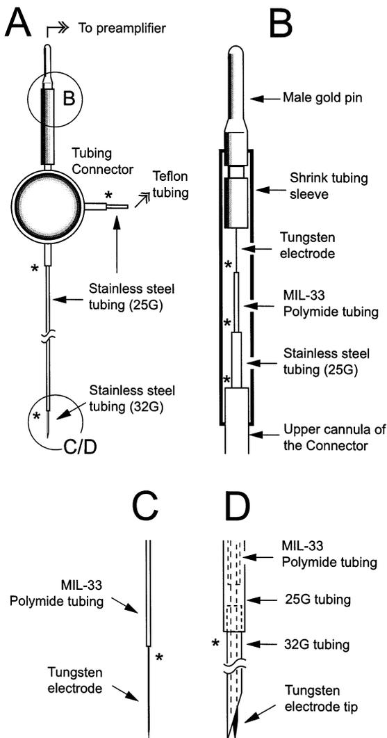
Fig. 1. Assembled injectrode (A) and configuration of the parts in detail (B–D). Asterisks indicate the places where a soldering job or epoxy glue is needed in order to seal the gaps at the junction.
