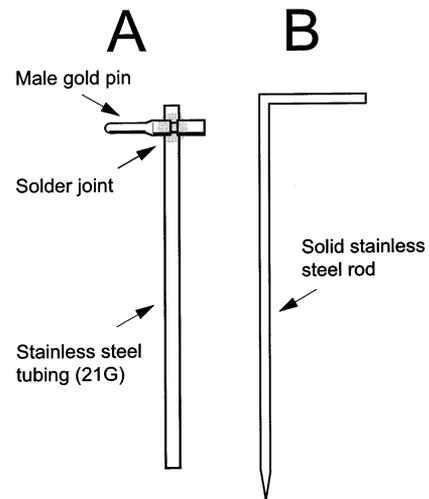
Fig. 2. Removable stainless steel guide tube (A) for fitting the injectrode, and dura-puncturing rod (B).
